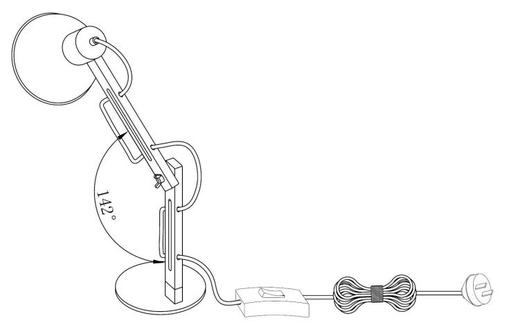
NOTE: When adjusting the upper arm (C), do not adjust more than 142° as this may damage the wiring.
