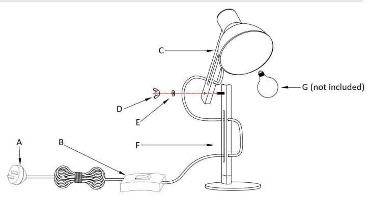
NOTE: Never adjust the upper arm (C) without first loosening the locking knob (D).
