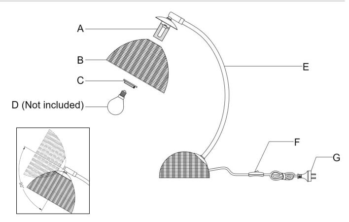
NOTE: When adjusting the lamp head (B), do not adjust more than 90 degrees shown in above diagram, as this may damage the joint and internal wires.
