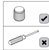
To avoid damage to the coin caps, always fasten using the plastic tool provided.
