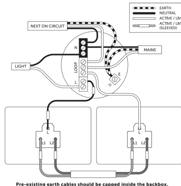
Pre-existing earth cables should be capped inside the backbox.
