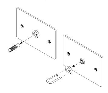
Connect the wires as shown in the appropriate wiring diagram. Use red or brown sleeving to mark cables used for ACTIVE or SWITCHED ACTIVE connections.
