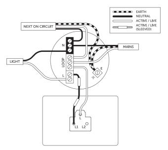
Pre-existing earth cables should be capped inside the backbox.
