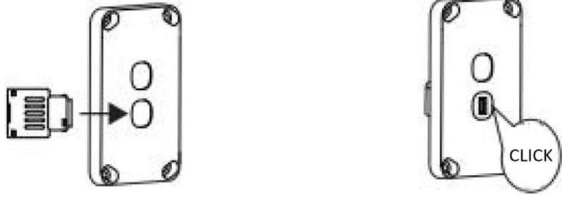
3. If you need to remove the USB mech, carefully and slowly pry it using a 4mm flat head screwdriver.
