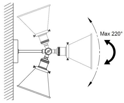
NOTE: Do not adjust the shade (J) more than 220°, as this may damage the knuckle joint or the internal wiring.
