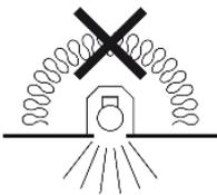
A recessed luminaire that can be used where normally flammable materials, including building insulation, are or may be present, but cannot be abutted against any material and cannot be covered in normal use.
