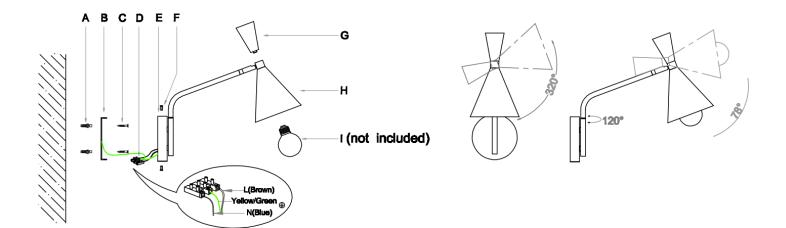
NOTES FOR ARM AND HEAD ADJUSTMENT: To avoid and damage to the joints or internal wiring, please do not adjust the arm or head beyond the angles listed:
