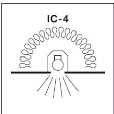
1. A closed luminaire that allows building insulation to come into contact with its sides and to cover it.
