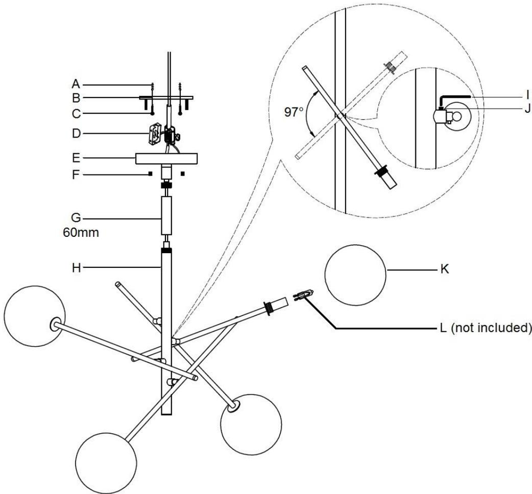
**NOTE:** Do not adjust the angle of the arm without first loosening the grub screw (J) with the allen key (I) provided, as this may damage the locking mechanism and will void warranty.
