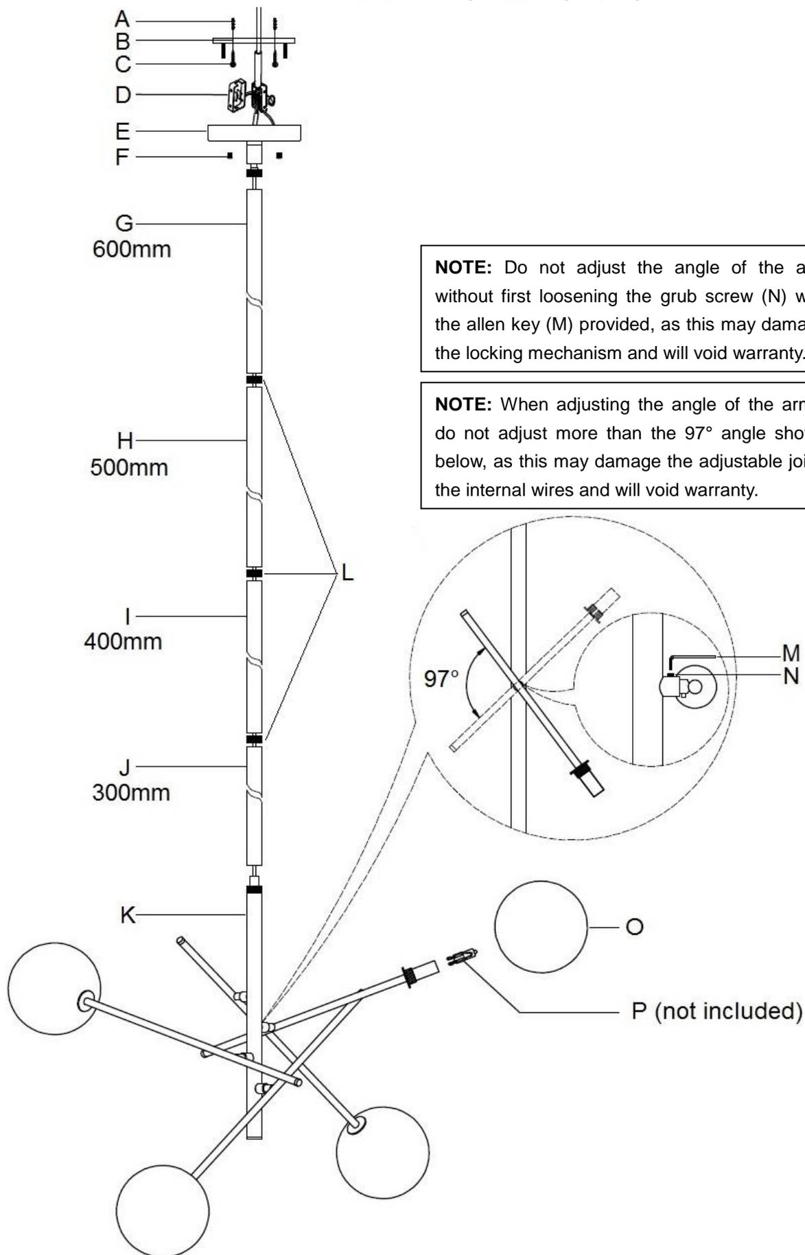
**NOTE:** Do not adjust the angle of the arm without first loosening the grub screw (N) with the allen key (M) provided, as this may damage the locking mechanism and will void warranty.
