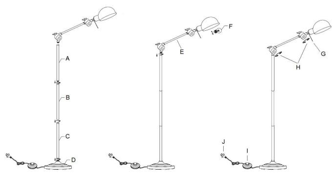
NOTE: When adjusting the arm or the head of the fitting, do not adjust more than 120° as this may damage the internal wires.
