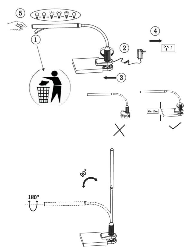
**NOTE:** When adjusting the angle of the head, do not rotate more than 180°as this may damage the internal wi res. When adjusting the height of the head, do not adjust more than 90°as this may damage the inter nal wires.
