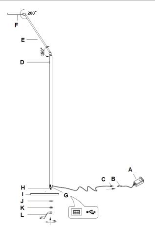
NOTE: When adjusting the rod (E), do not adjust more than 180° as this may damage the internal wires.
