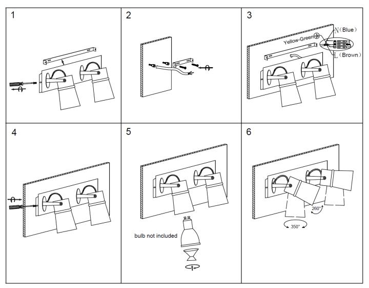
Note: When adjusting the spot lights, do not adjust more than the angles shown in figure 6 as this may damage the internal wiring and void the warranty.
