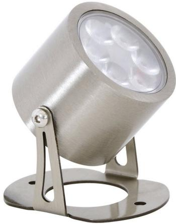
The Sentinel 12V pond light is rated as IP 68 and is great for use in a pond that is no deeper than 2m. The Quick connectors are rated as IP65 and need to be protected from continuous immersion water, ensure there is adequate drainage around the connectors so that water does not pool around them. The Sentinel pond light comes with 4m of cable.
