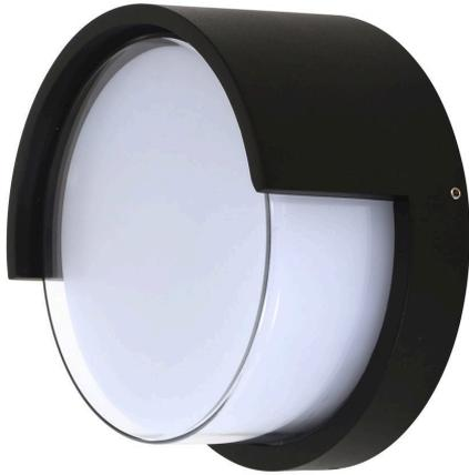
The Remius Bunker range produces a beautiful diffused light, perfect for lighting up porches or alfresco areas. The Remius is made from die cast aluminium with ABS plastic diffuser and is able to colour switch from, 3000K-4000K. It is IP65 rated with a 450 lumen output of light. The Remius is non dimmable and must not be installed on a circuit which has a dimmer switch.
